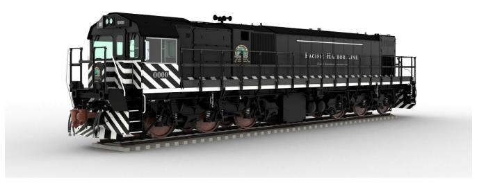
The zero-emission, zero-idle and low noise EMD® Joule locomotive, capable of 3,200 horsepower in this application, will be rigorously tested in all types of service at PHL.
