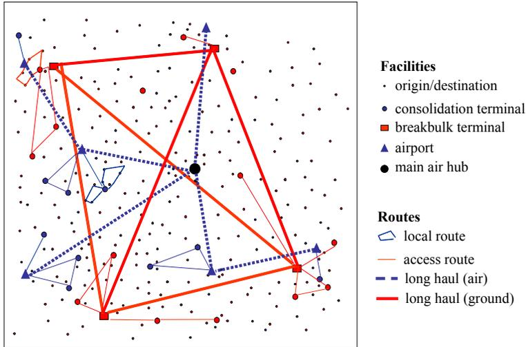
Figure 1: Integrated package distribution network
