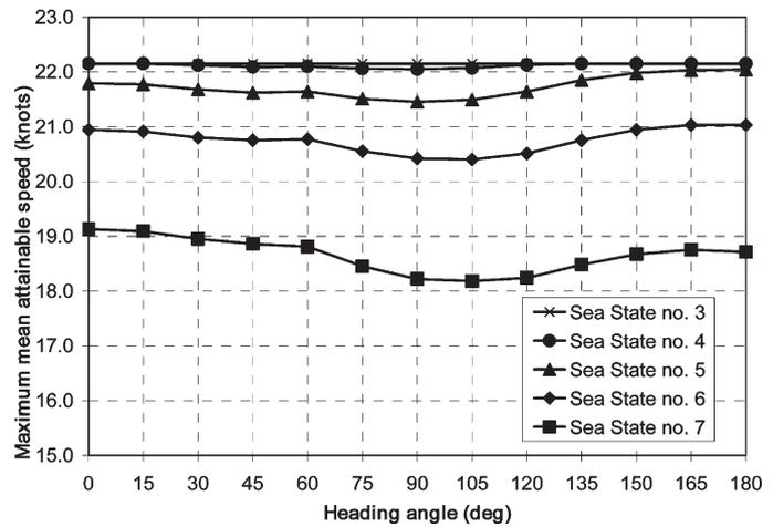
Fig. 1 Maximum mean attainable speed for S-175 as a function of ship relative heading angle and sea state
