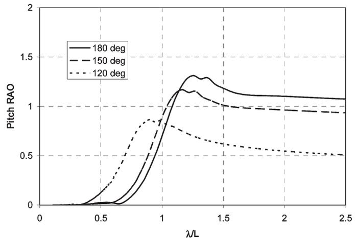
Fig. 3 Pitch RAO at  $F_n = 0.275$  for S-175 as a function of ship relative heading angle
