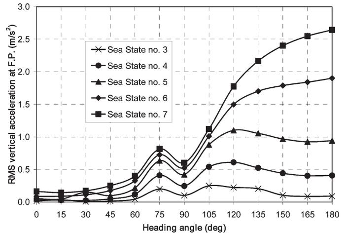
Fig. 8 RMS vertical acceleration at the F.P. for S-175 as a function of ship relative heading angle and sea state
