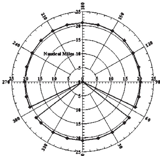
Fig. 11 Constrained linear path attainable regions for the S-175 for Sea State 6
