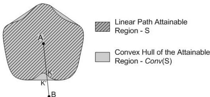
Fig. 13 Computing bound on an optimal travel time for nonconvex attainable region
