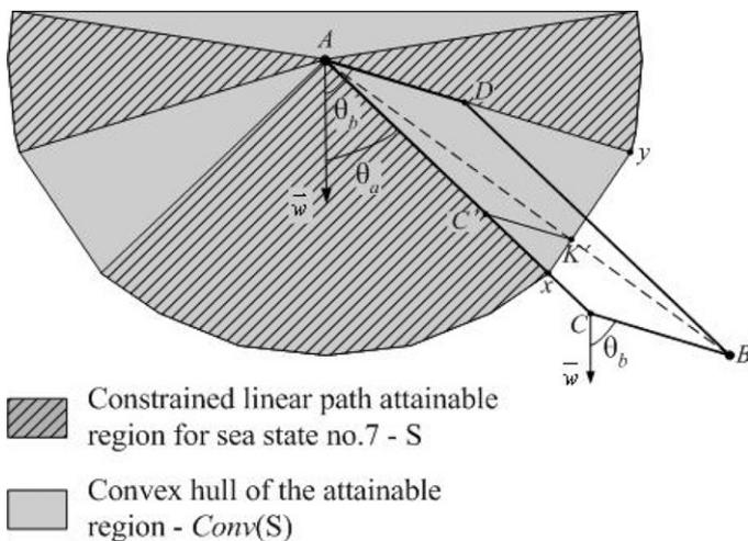
Fig. 14 Fastest paths from  $A$  to  $B$  are  $ACB$  and  $ADB$
