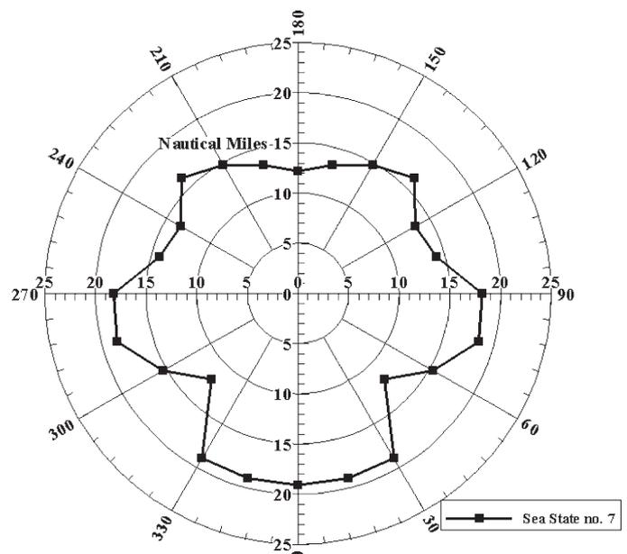
Fig. 16 An example of linear path attainable regions for the S-175 corresponding to voluntary speed loss at Sea State 7
