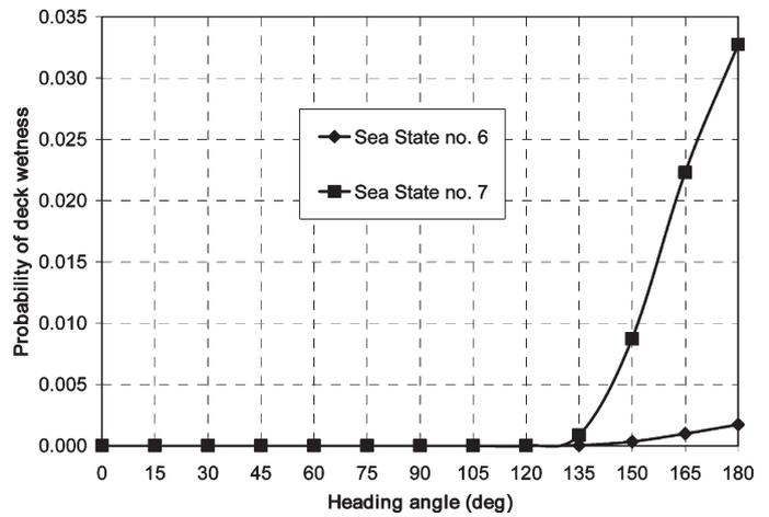
Fig. 6 Probability of deck wetness for S-175 as a function of ship relative heading angle and sea state
