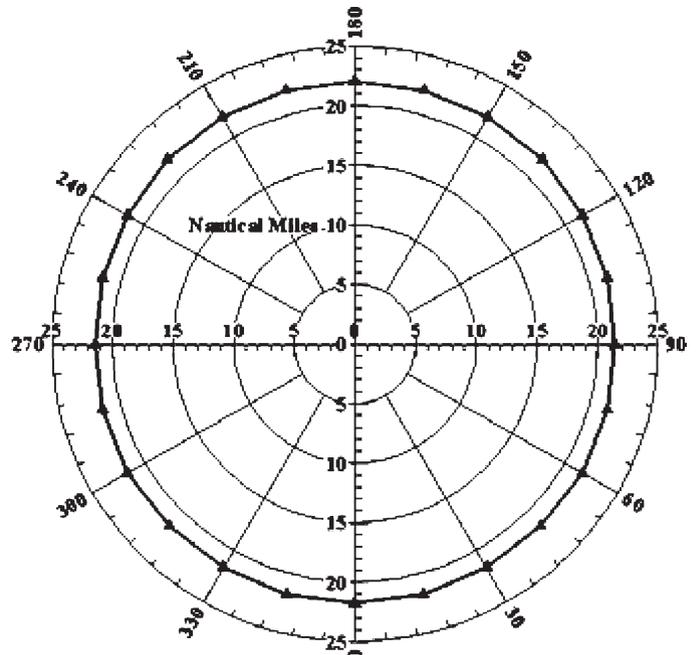
Fig. 10 Constrained linear path attainable regions for the S-175 for Sea State 5
