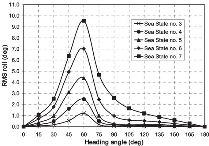
Fig. 4 RMS roll for S-175 as a function of ship relative heading angle and sea state
