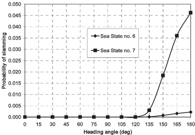
Fig. 5 Probability of slamming for S-175 as a function of ship relative heading angle and sea state
