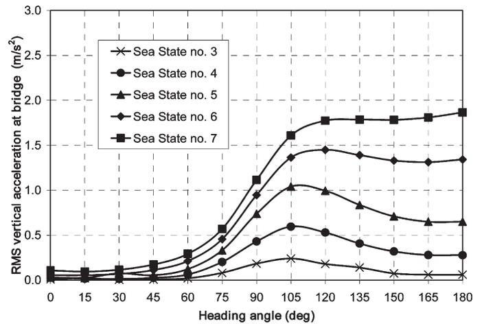
Fig. 7 RMS vertical acceleration at the bridge for S-175 as a function of ship relative heading angle and sea state
