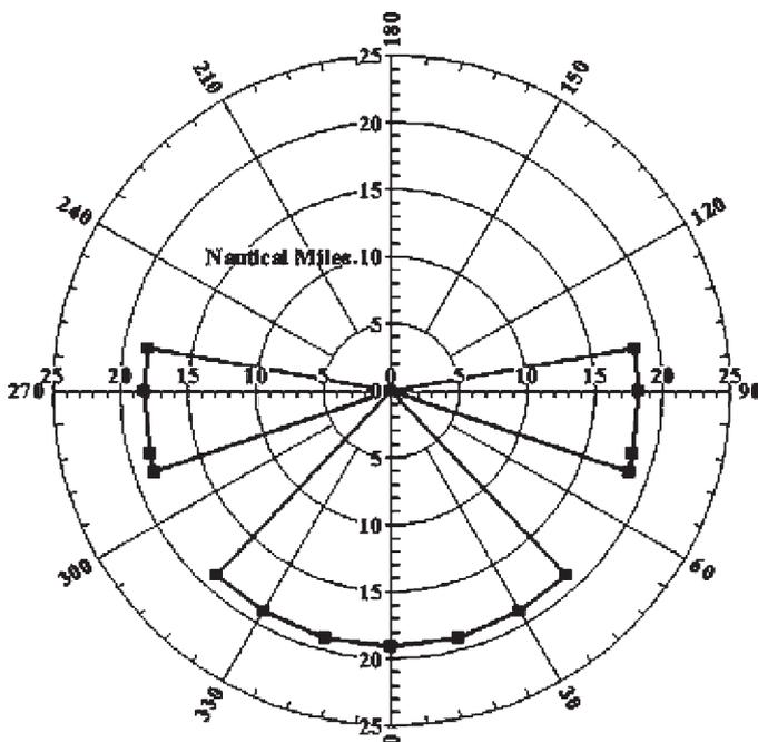
Fig. 12 Constrained linear path attainable regions for the S-175 for Sea State 7
