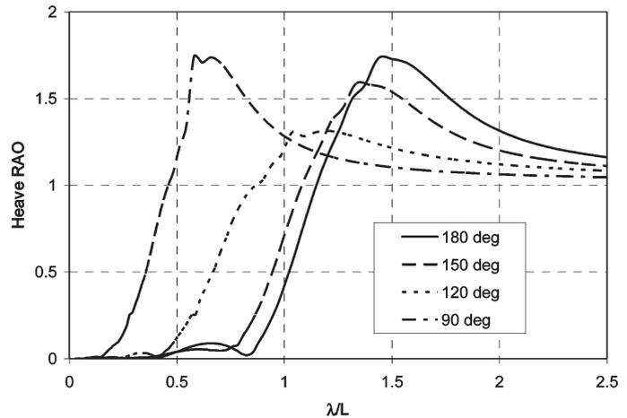
Fig. 2 Heave RAO at  $F_n = 0.275$  for S-175 as a function of ship relative heading angle
